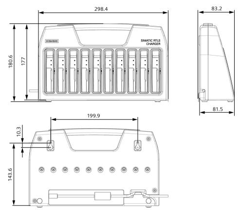
Figure 2-2 Dimension drawing of SIMATIC RTLS charging station (not included with the product) - All dimensions are given in millimeters
