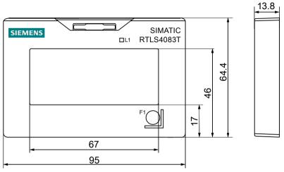
Figure 2-1 Dimension drawing of SIMATIC RTLS4083T - All dimensions are given in millimeters
