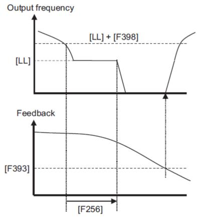
This diagram shows the output frequency falling below the <LL: Lower Limit frequency>. The output frequency would go into the sleep state after running for a duration based on <F256: Run Sleep detection time>. The second graph shows the time interval during the operation. The AS3 will wake up based on the <F393: Wakeup feedback> and the output frequency will increase based on the demand of your application.
