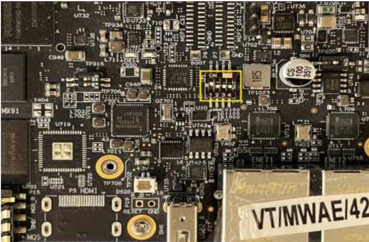
Figure 7. Boot mode selection switch
