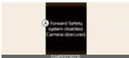
A: Forward safety system disabled. Camera obscured
