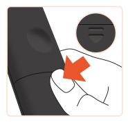
**1.** Press and hold your thumb on the arrow to release the latch.
