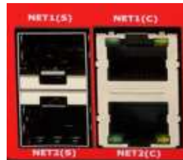
Figure: Network interfaces for OM1200
