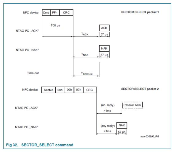
Changes active memory sector which is accessed by read/write Note: second part of command has a passive ACK – no response is ACK!
