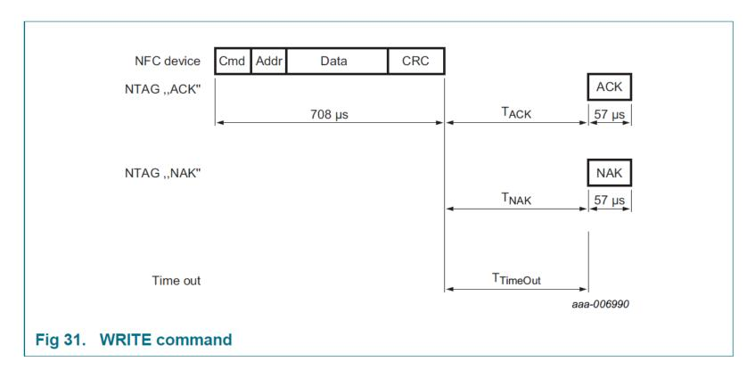
WRITE command needs page address and 4 bytes of data as parameters
