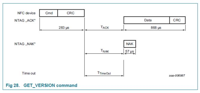
Provides 8 byte of identification data to exactly identify which NXP-IC it is
