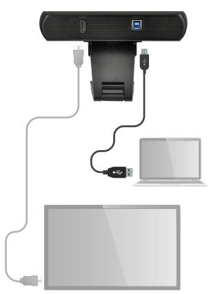
**Note:** starting from version 8.4.037, the HDMI port is disabled by default. It is possible to enable it through the camera "Setting" menu that can be recalled in overlay using the camera remote control and pressing the menu button.
