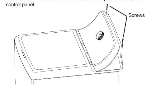
Grasp the control panel sides, push it back, and roll it toward the rear so the pressure sensor tube can be seen where it connects to the control
