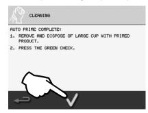
Press the green check to continue to the Sanitizing Ice Bin & Water Nozzles screen. If this feature is not turned on in the Managers Menu, proceed to "Blenders / Dispense Area Cleaning & Sanitizing" on page 46.
