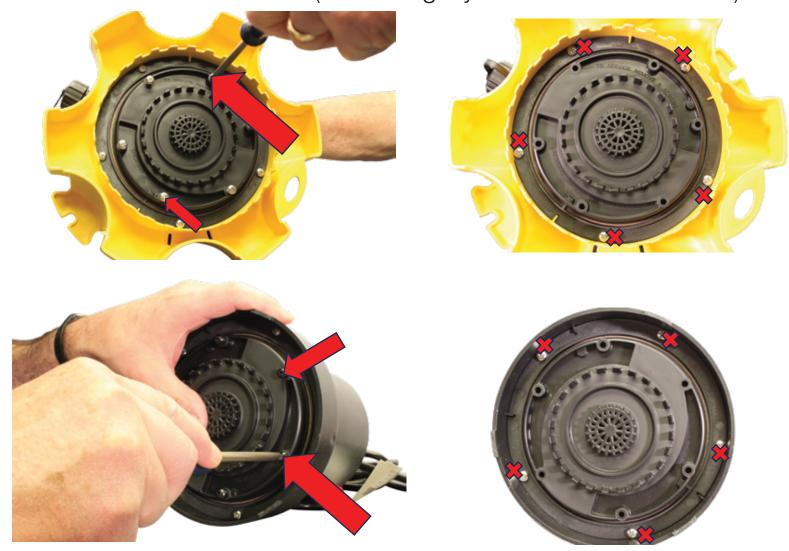
4. Using care to not tear the cork gasket on the bottom side of the inlet screen, gently separate the inlet screen from the pump. Clean and rinse any debris from the inlet screen.
