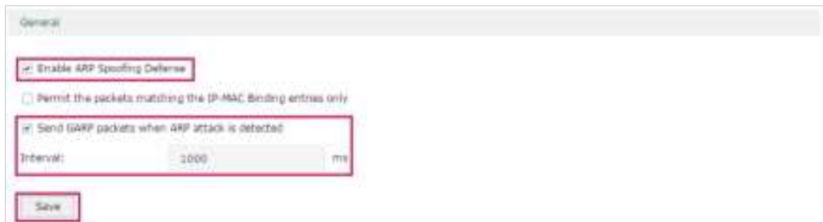
Figure 3-5 Configure Anti ARP Spoofing
