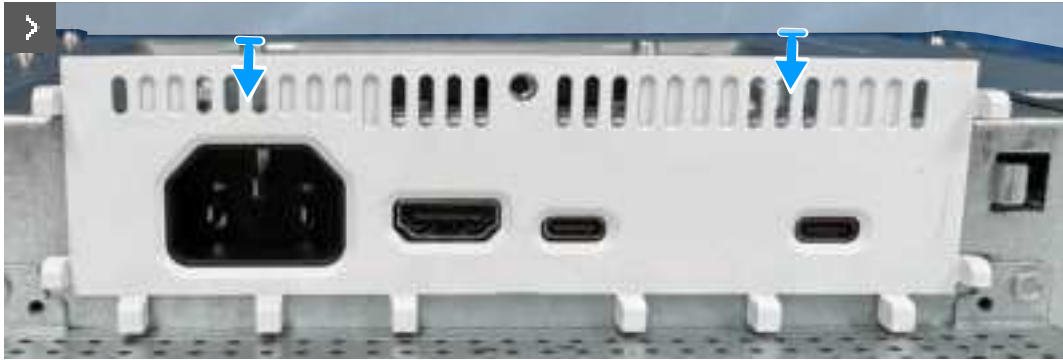
Figure 16. Removing the metal shield I/O-cover
