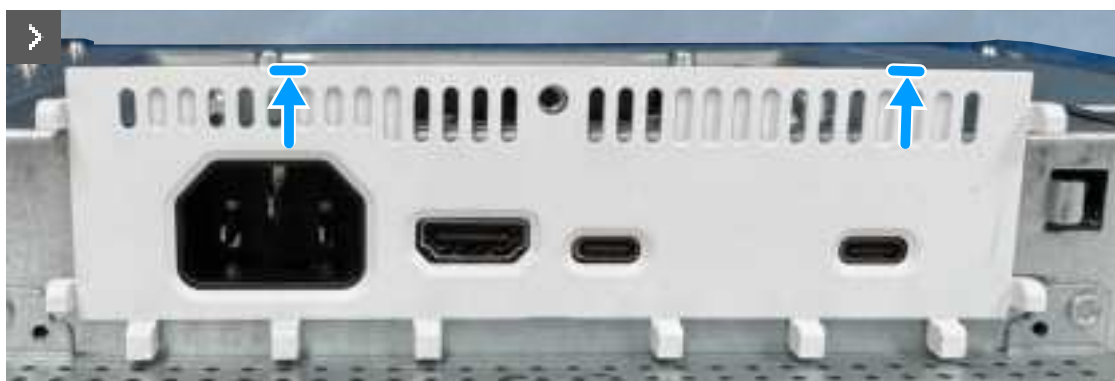
Figure 21. Replacing the metal shield I/O-cover
