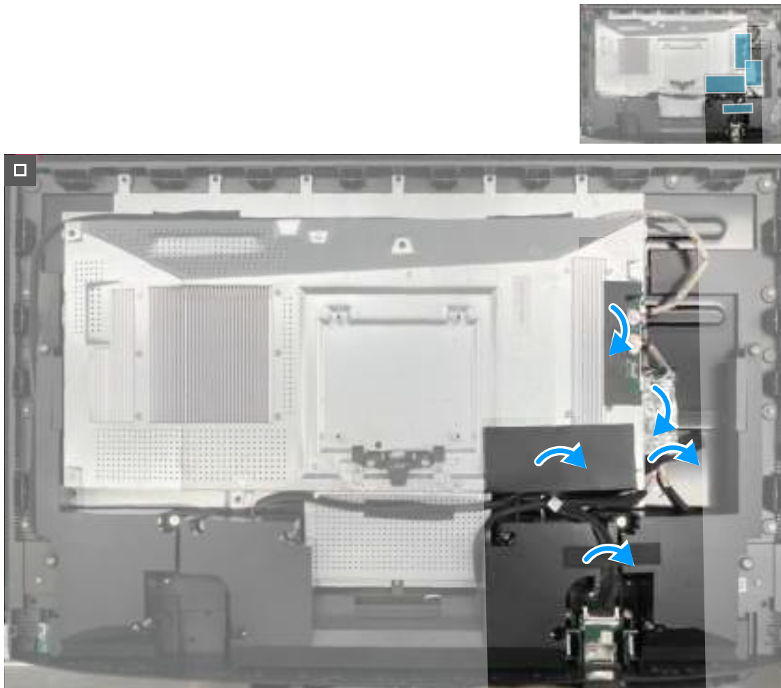
Figure 10. Adhere the tapes and Mylar to secure the cables and metal shield
