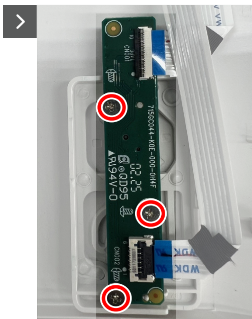
Figure 29. Removing the keypad board and disconnecting the cables
