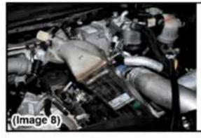
Step 12: Hold the intercooler tube back while pulling the vertical EGR cooler up and out. You may have to rotate the cooler to release it from its mount. (Image8)
