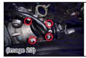
Step 37: Remove four bolts and loosen hose clamp on the intercooler plumbing to remove the EGR valve. (Image 23)
