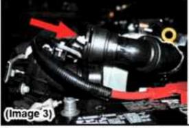
Step 5: Remove the upper radiator hose by popping the wire clip out and pulling the hose straight out. (Image 3)
