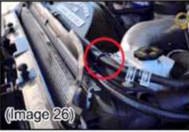
Step 40: Secure the coolant line over the radiator with the plastic hose routing clips. (Image 26)
