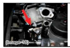
Step 27: Remove the coolant tube that was conneced from the vertical EGR cooler to the engine. Replace it with the coolant plug supplied in the kit to block off the hole. (Image 18)
