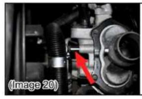
Step 29: Use 13mm wrench to Re-install the stud using the spacer provided in the EGR delete kit. Then secure the power steering line to the stud.(image 20)
