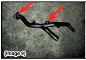
Step 13: Remove the plastic coolant tube.Be careful to not break the coolant tube as it will be re-used during installation.(Image 9)
