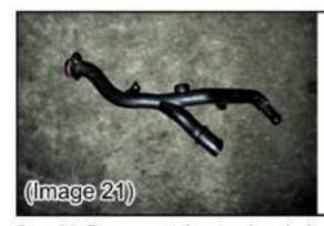
Step 30: Re-install the plastic coolant tube. Be careful not to crack or break it.(Image 21)
