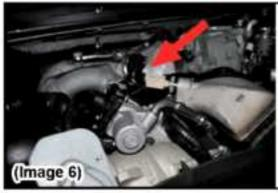
Step 10: Disconnect the electrical connector on top of the vertical EGR cooler.(Image 6)
