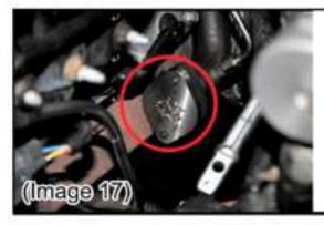
Step 25: Install the exhaust block off using M10-1.125 x 20 bolts and gasket. (Image 17)
