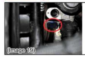
Step 28: Install the coolant plug included in the EGR delete kit. Use the factory bolts that secured the lines in place. (Image 19)
