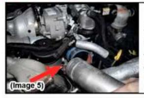
Step 9: Loosen the clamp on driver side intercooler tube and separate the intercooler tube from the rubber boot. It is not necessary to remove the tube.(Image 5)
