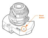
Resetting the camera: To reset the camera, use the tip of a paper clip or a pencil and press the reset button. Pressing the button for five (5) seconds will initiate a camera-wide reset of all the settings, including network settings.
