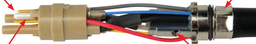
Pins Properly Crimped & Inserted
