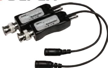
Supports SMPTE-424M (3G-SDI), SMPTE-292M (HD-SDI), and SMPTE-259M (SDI) specifications • Extends 3G-SDI up to 1.25 miles (2 kilometers) over one single-mode ST-terminated fiber optic cable
