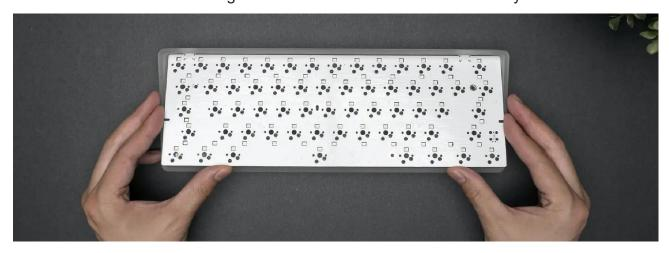
After, grab your brass standoffs, thread and tighten them by hand through each of the four holes into the inserts below.
