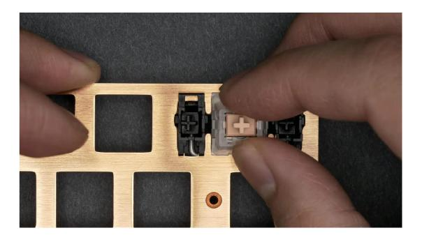
Next, place the plate over the PCBA and make sure the switch pins are aligned with the hotswap sockets. Press down on opposing corners to seat the switches.
