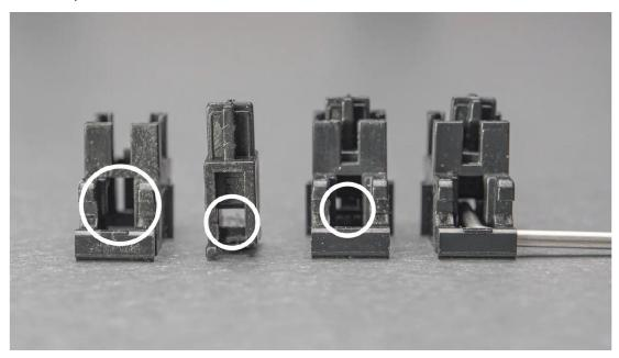
If it refuses to go in all the way, the wire was placed too high up on the insert. Pull the wire out, raise the insert and try again.
