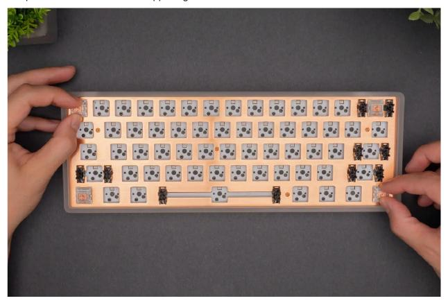
Take your screws and secure the plate through the four holes. Start from the middle screw and work outwards so the pressure is evenly distributed.
