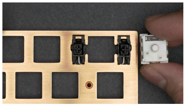
Align each switch so the pins line up with the hot-swap socket. To insert, center the switch over the plate. You want to make sure all sides are level so the pins can easily slide straight into the socket. Using two fingers push straight down with even pressure to seat the switch. It will clip into the plate.
