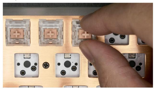
Repeat this same process across most of the board, checking the pins are straight each time. It is recommended that you install switches starting from the ends of each row and work your way towards the middle of the row.
