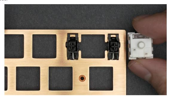
To insert the four switches in each corner, center each switch over the plate, ensuring that the pins align with the sockets, and press firmly until seated. They will snap into place.
