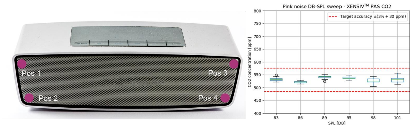
Figure 7 Acoustic robustness of XENSIV™ PAS CO2
