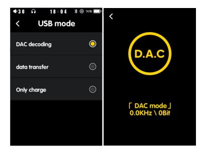
Turn on the player, go to system setting, set USB mode at DAC decoding, and then connecting to PC, and then you can see PC shows "find new hardware", no need any operation, it will automatically install.
