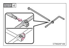
Assemble the jack handle and tighten the screw.
