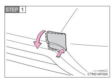
Remove the eyelet cover while pushing it.
