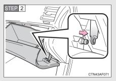
Open the glove box. Slide off the damper.
