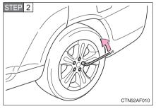
Slightly loosen the wheel nuts (one turn).
