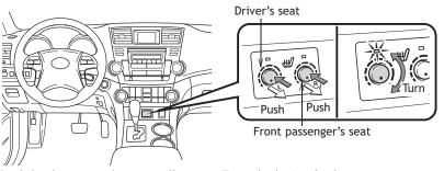
Push knob to pop the controller out. Turn clockwise for heater.
