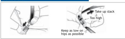
If belt is fully extended, then retracted even slightly, it cannot be re-extended beyond that point, unless fully retracted again. This feature is used to help hold child restraint systems securely.
