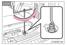
Connect the jack handle and the adapter socket. Turn the jack handle.
