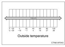
Recommended oil viscosity (3.5 L V6 (2GR-FE) engine)
