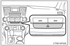
Press the switch to flash all the turn signal lights. To turn them off, press the switch once again.
