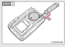
Remove the depleted battery.
