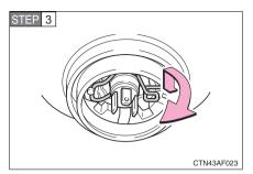
Release the bulb retaining spring.
