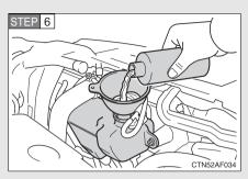
Add engine coolant if necessary.
