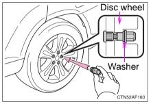
Turn the nut washers until they come into contact with the disc wheel.
