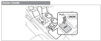
The snow mode prevents sudden acceleration on slippery surfaces. Use in snowy or icy road conditions.
