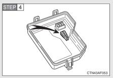
Remove the fuse with the pullout tool.
