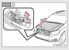
Lift the auxiliary catch lever and lift the hood.
