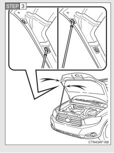
Hold the hood open by inserting the supporting rod into either of the slots.
