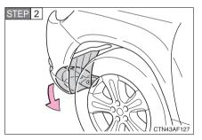
Remove the fender liner.
