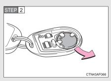
Remove the discharged transmitter battery.
