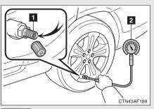
STEP 1 Remove the tire valve cap.
