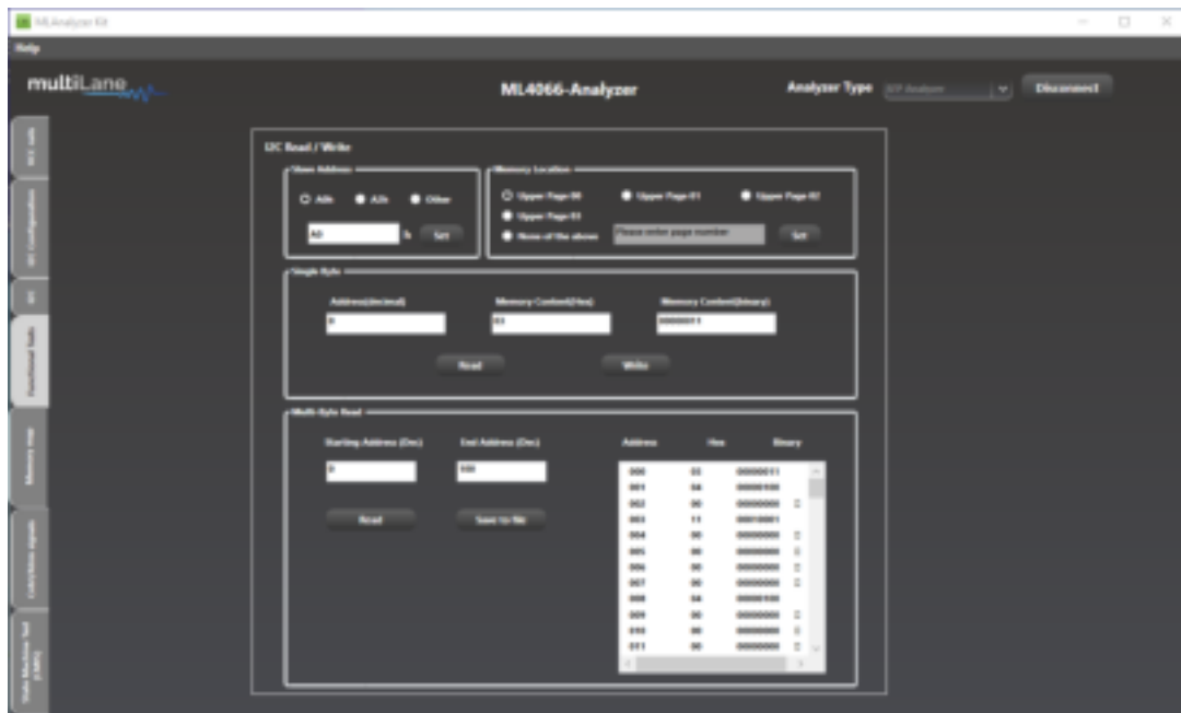
Figure 14: Reading Specific Registers from Functional Tests Tab
