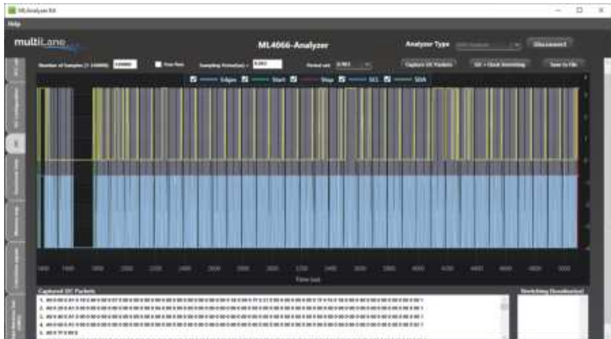
Figure 3: I2C Capture tab
