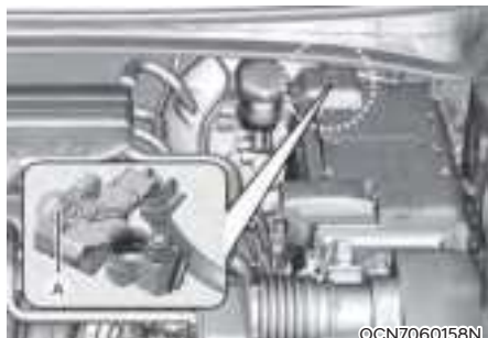
[A] : Battery sensor
