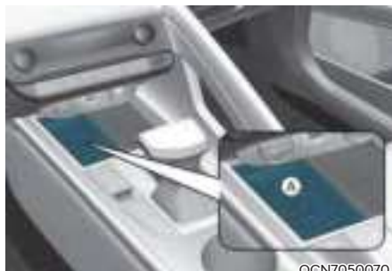
[A] : Wireless Charging Pad (In-vehicle Authentication Pad)
