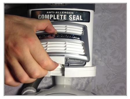
Press up on the latch and remove the front vent
