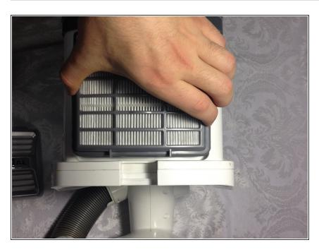
Lift the HEPA filter out of the vacuum
