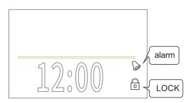
Alarm: Press "ENTER" button and "MINUTE" button together can activate/deactivate the alarm. It will be on when countdown runs up. Pressing any button can stop the alarm.
