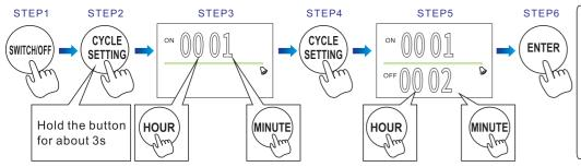
Hold "CYCLE SETTING" button for 3 seconds, the upper digits will flash. The digits on the left is for minutes, and can be set using the "HOUR" button: the digits on the right is for seconds, and can be set using the "MINUTE" button
