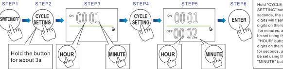
SETTING" button for 3 seconds, the upper digits will flash. The digits on the left is for minutes, and car be set using the "HOUR" button; the digits on the right is for seconds, and can be set using the "MINUTE" button.
