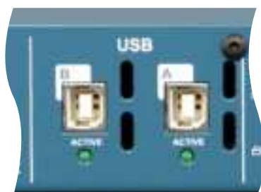
ACTIVE LEDs indicate connection to each computer
