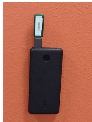
Attach Range Test node on wall
