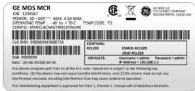
Figure 8, above: Orbit MCR Label showing “Contains E5MDS-RCL220, 101D-RCL220”
