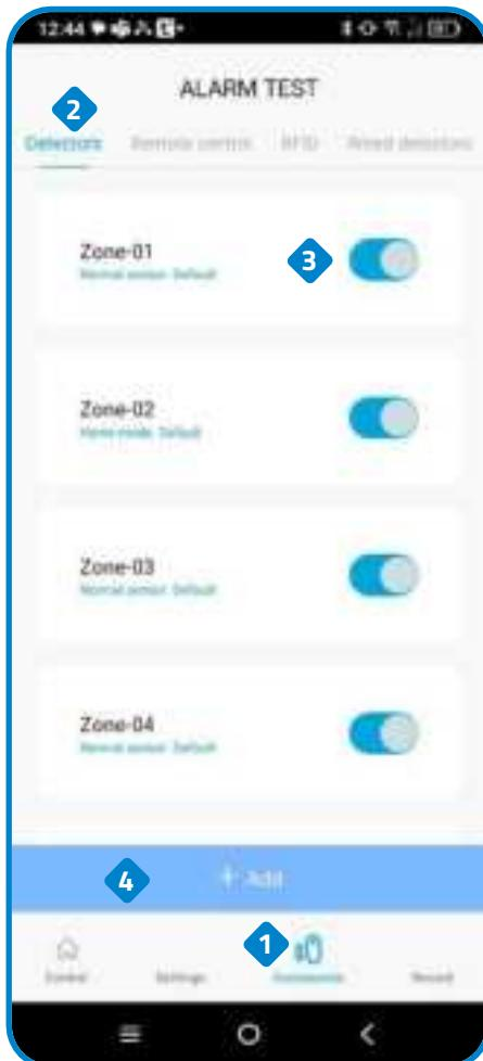
3 Allows to activate or deactivate a previously added sensor or zone.
