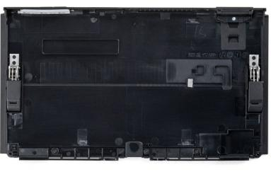
• Use Phillips driver to remove the four 2.1 mm screws securing the kickstand to the rear case.
