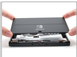
Lift the rear case up from the top of the device and remove it.
