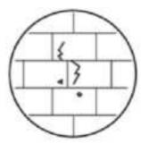
Take extra care when drilling into high walls or ceramic tiles. Wall anchors should be a tight fit for the hole. Never use wall anchors in ceilings.
