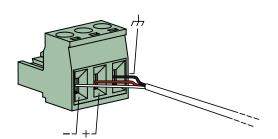
For unbalanced line input connections.
