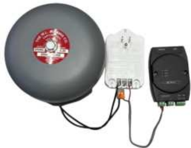
Netbell-2 Wiring Sample
