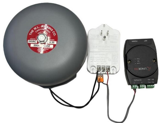
Netbell-2 Wiring Sample
