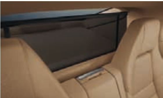
Retractable luggage compartment cover with electric roll-up sunblind for behind the rear compartment
