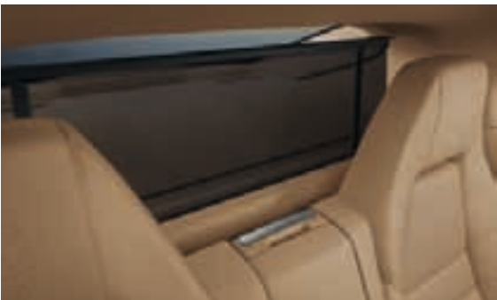
Removable luggage compartment cover with electric roll-up sunblind for behind the rear compartment
