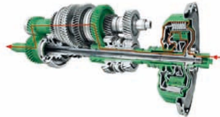
Power flow in 2nd gear
