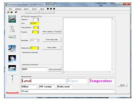
Optilevel probes are working at 9600 bauds but if they have never been configured, they are at 300 bauds (use settings/communication menu to set the correct bauds rate).
