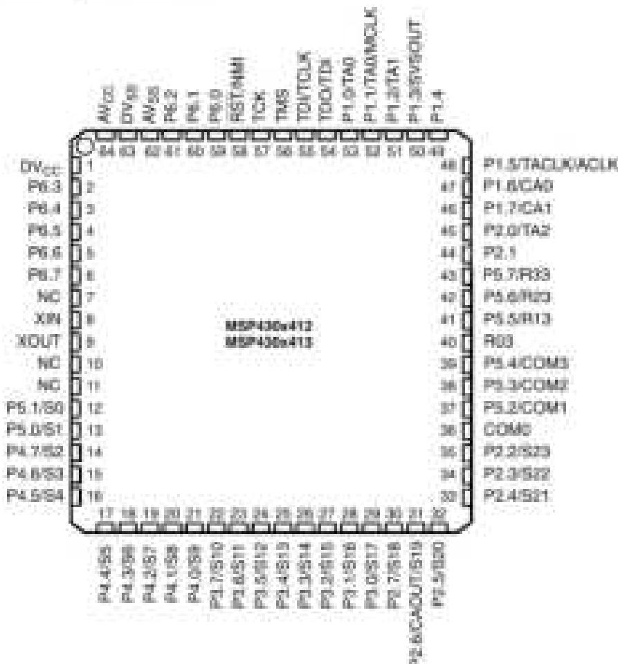
NC = No internal connection. External connection to V<sub>DD</sub> recommended.
