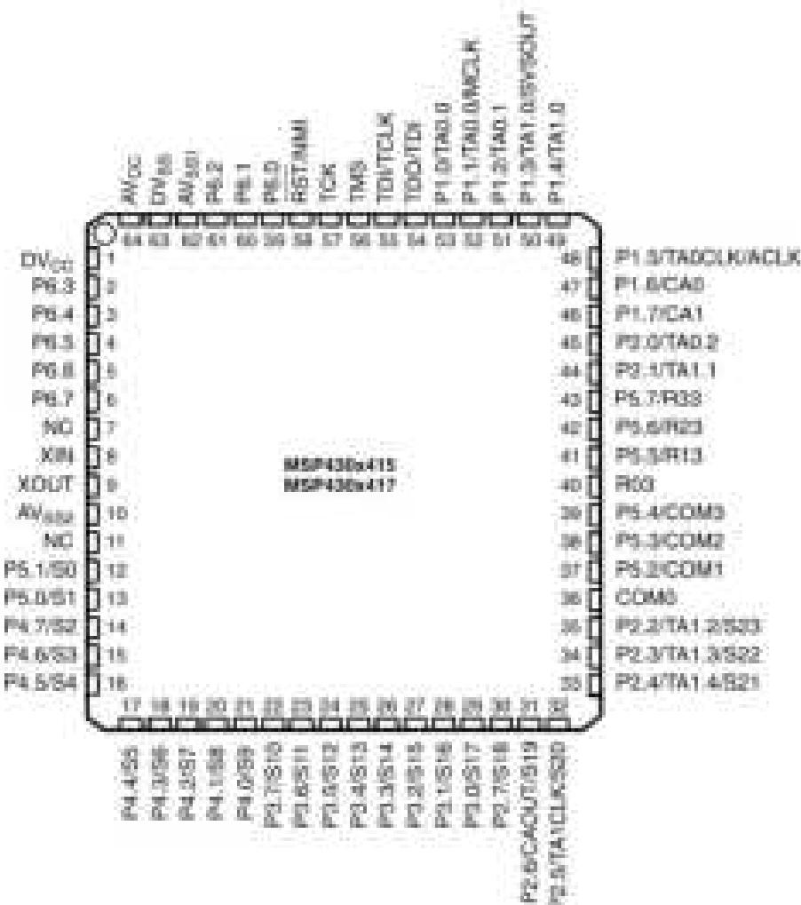
NC = No internal connection. External connection to V<sub>SS</sub> recommended.
