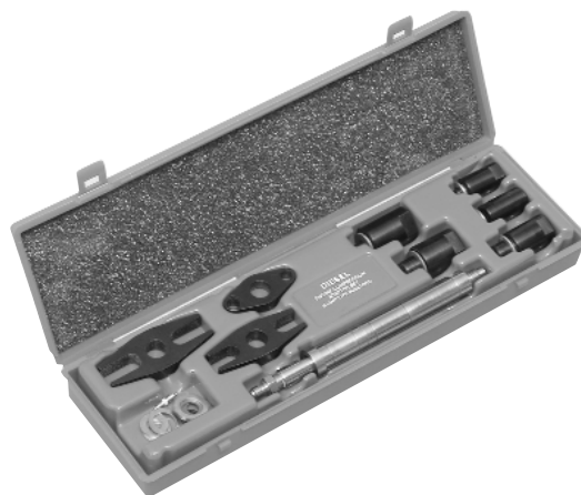
Claw held injectors - use the actual injector clamp NOTE: Use large diameter Spacer in top position for wider claws
