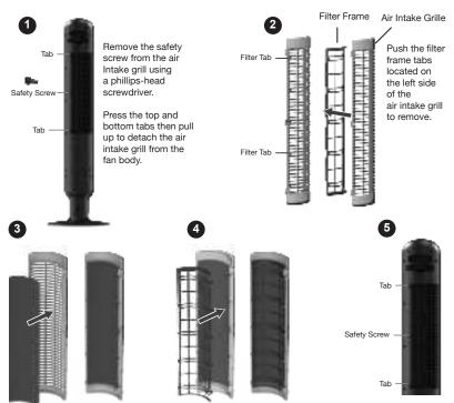
Place the filter inside of the air intake grille.
