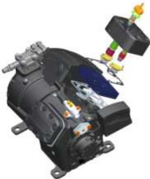
Figure 2: Exploded view of the digital mechanism
