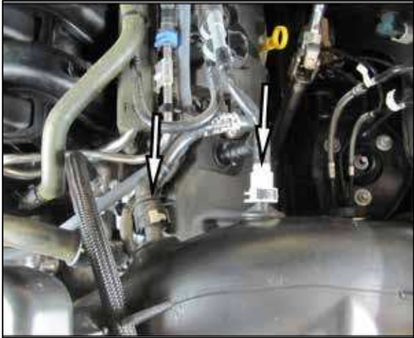
3. Disconnect the two breather lines and remove the intake tube from the vehicle.
