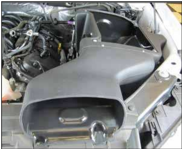
10. Place the Airaid air Box/Inlet assembly into the inner fender area of the vehicle as shown.
