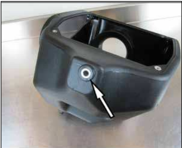
7. Insert the 5/8" Grommet and Spacer into the opposite side of the Airaid Air Box.
