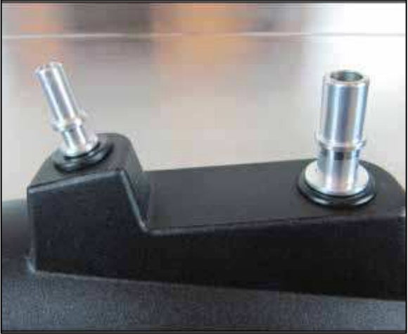
14. Gently insert the Aluminum Breather Fittings into the Grommets. Hint: Soapy water makes for a good Grommet lube .
