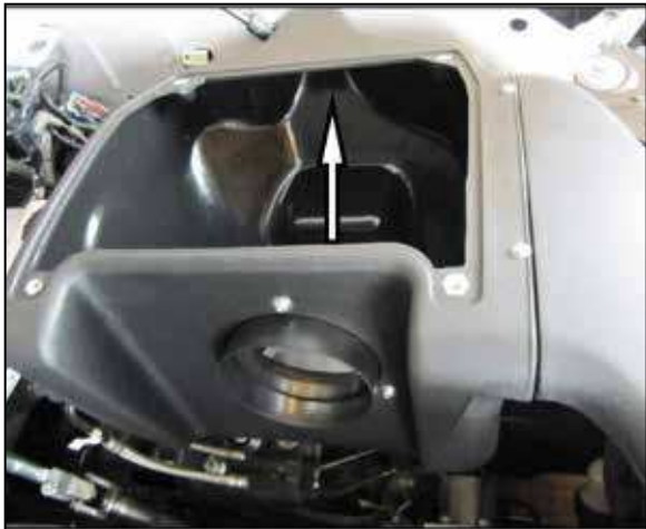
12. Secure the Airaid Air Box to the inner fender using the 8mm bolt removed in step 5. NOTE: on vehicles that have a wiring harness that was attached to the engine side of the factory air filter housing, find a suitable location (above the tube and below the top of the AIRAID cold air box) and drill two 1/4" id holes. Using the provided mounting tie wraps, secure the wiring harness to the cold air box.
