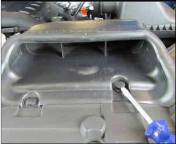
4. Using a standard blade screwdriver, gently pry up the center posts of the plastic rivets in the air inlet and remove them.
