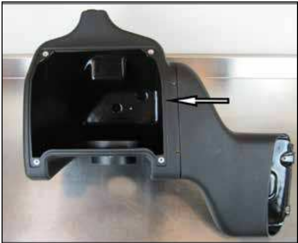
8. Snap the new Air Scoop into the Airaid Air Box as shown.
