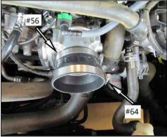
15. Slide the Reducing Coupler and Clamps onto the throttle body as shown. The Small end will use the #56 Clamp and the Large end is to use the #64 Clamp.
