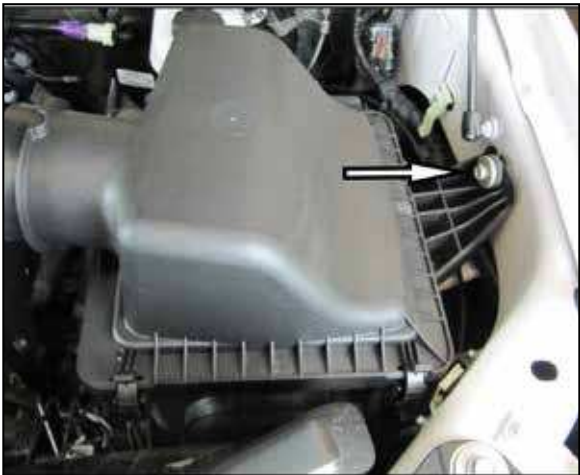
5. Remove the 8mm fender bolt in the air box and remove the entire air box/scoop assembly from the vehicle. NOTE: On vehicles equipped with a wiring harness attached to the airbox, be sure to unclip the wiring harness from the air box before removal.
