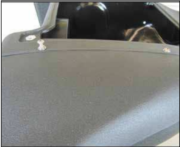
9. Secure the Scoop to the AirBox using the two sets of 8-32 Button Head Screws, Lock Washers and Flat washers.
