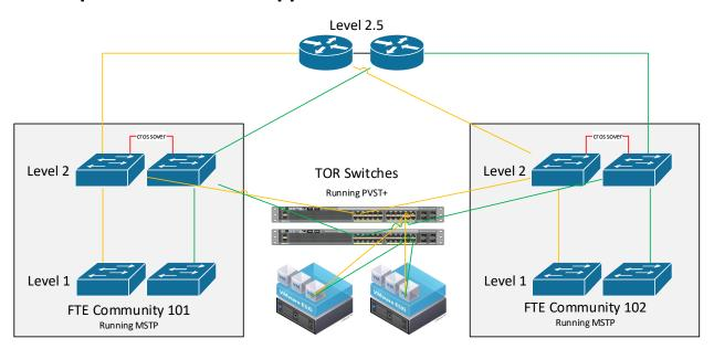
Before integrating the Top of rack switch into the FTE Community each FTE community switch must have **root guard** implemented on each of the TOR switch connections.
