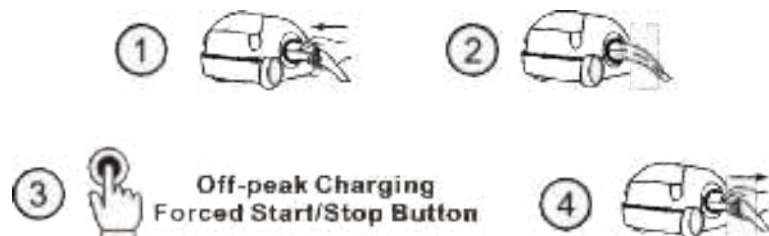
Plug&Charge mode operation process flow
