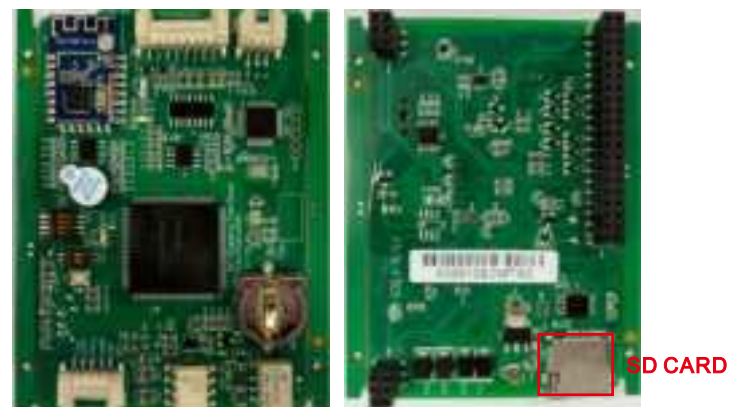
Micro SD slot of 22kW charger
