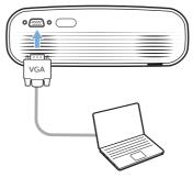
On your computer, adjust the screen resolution of the computer to the correct setting and switch the VGA signal to an external monitor. The following resolutions are supported:
