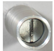
Fully Engaged Latch
