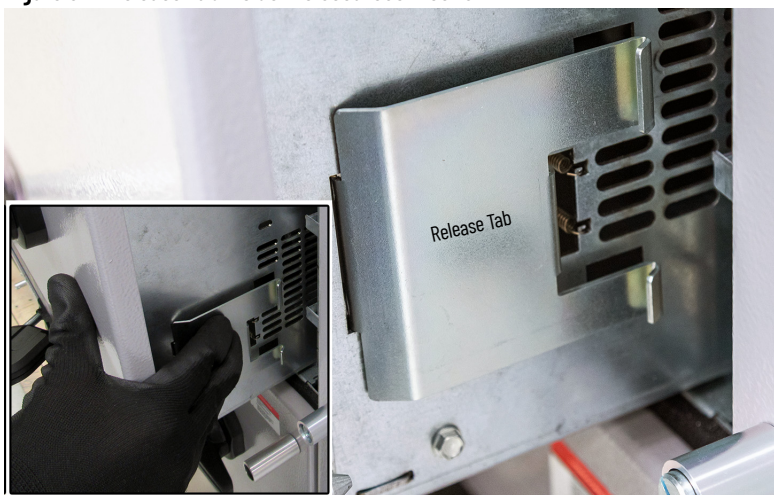
Figure 32 - Release Tab Inside the SecureConnect Unit
