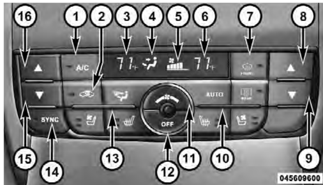
Automatic Temperature Control (ATC) Panel
