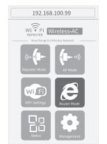
6 Select PPPoE (ADSL dialing) for Internet Access. Then please input the broadband name and password correctly, which is provided by your network provider. Set a wifi name and password for the wifi extender.
