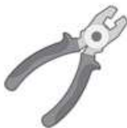
Wire-stripping tools for stripping 6-AWG copper wire
