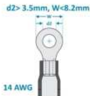
14-AWG wire with ring terminal for DC power supply
