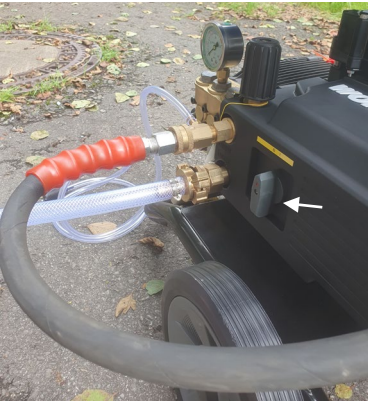
Fig. 37: Rotary switch marked with an arrow
