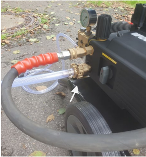
Fig. 29: Connection for the water supply marked with an arrow
