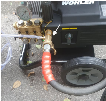
Fig. 28: Quick coupling on the motor marked with an arrow
