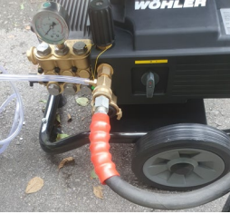
Fig. 42: Connection hose and air hose correctly fitted
