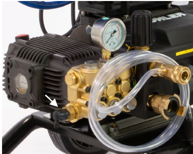
Fig. 44: Overpressure valve marked with an arrow
