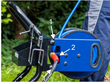
Fig. 27: Bolts on the drum holder marked with an arrow
