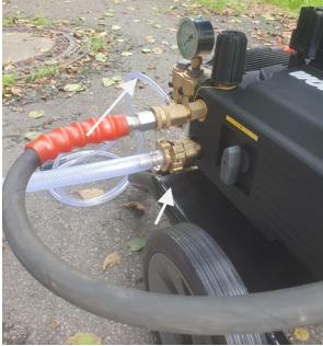
Fig. 43: Water supply marked with an arrow
