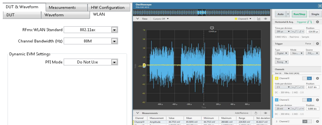
Figure 8: Scope Trace of RF and Enable Pulse without PFI
